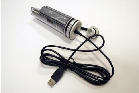
As one example of the way things are going, in the early days of CSP volunteers needed to take expensive (£2K) waterproof laptops up the hill to download water table data. This is no longer necessary as these have been replaced by HOBOTM shuttles (<https://www.tempcon.co.uk/shop/data-loggers/onset-hobo-data-loggers/hobo-dataloggers/hobo-u23-data-loggers>) which can download data via an optical interface (a memory stick which links wirelessly to a data logger). These pieces
