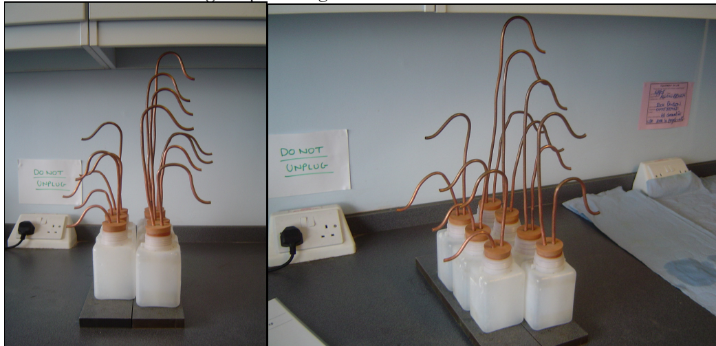
Figure 2: A rising-stage sampler with one tube for inlet and one tube for air exhaust. The intake tubes were positioned so that there was a few centimetres difference between them with the intention of taking samples at regular intervals.
