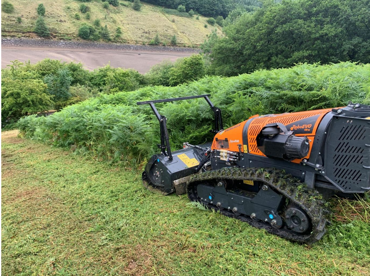
Figure 2. Remotely driven flail cutting plot I (TTFFI) for the first time in July 2022.
