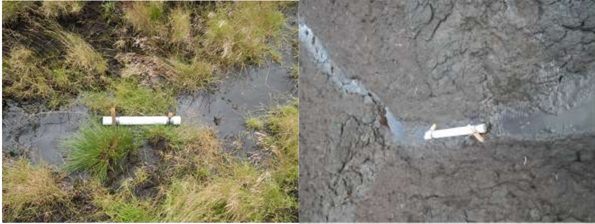
Fig. 1. TIMS units staked to the bottom of a re-vegetated (left) and an eroded gully (right).
