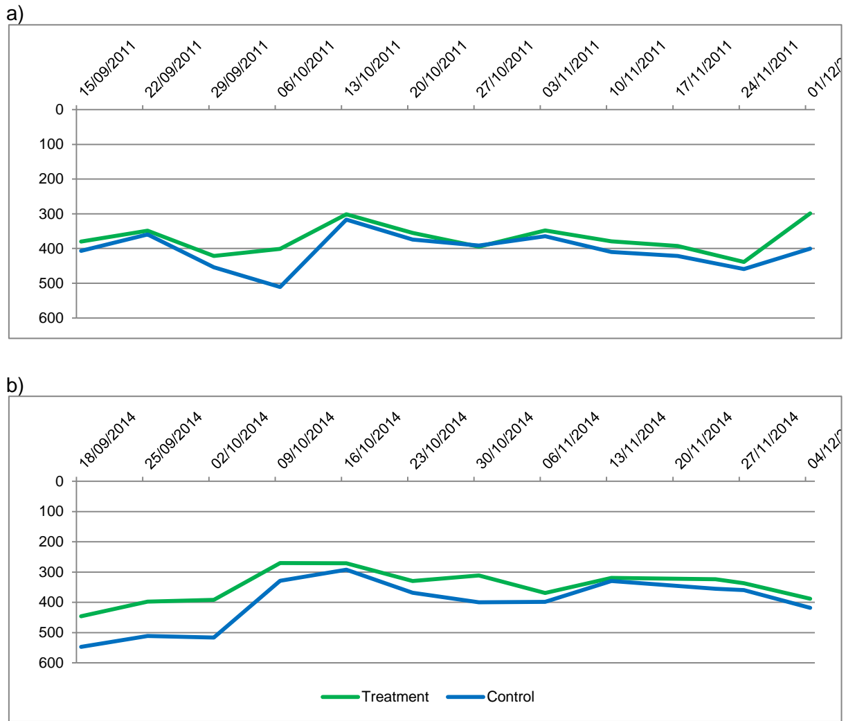
Figure 7 – Treatment and control comparison of depth to water table for Bleaklow study site
